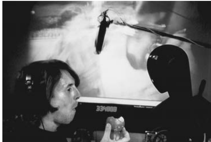
Right: Recording binaural Foley. Sound person eats apple in front of Aachen artificial head and attempts to match distance from camera and room acoustics with shot in 3D film being projected on video in background.
