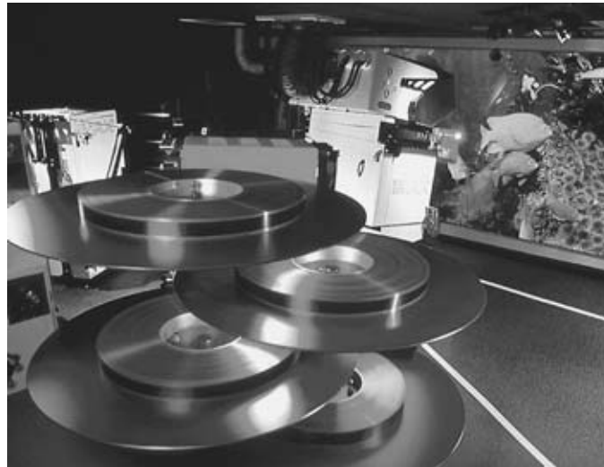
Right: Interior Of Projection Room, Fish From "Into the Deep" Visible On The Screen Through Glass Front Of Room. Large Platters Holding The Film Horizontally Are In Immediate Foreground. Photo: William Taufic
