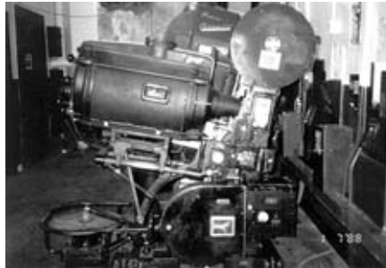
Figure 3: Early 1930s Simplex projector with sound-on-disc and sound-on-film capability.
