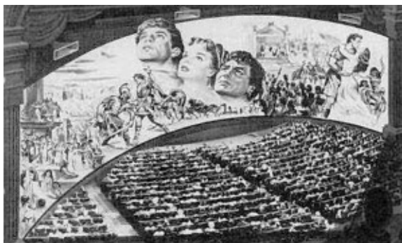
Figure 6: Diagram showing CinemaScope theater design, using one projector and three screen channels (the curvature of the screen in this drawing was absurdly exaggerated by Fox's publicity department to make it look like Cinerama's).
